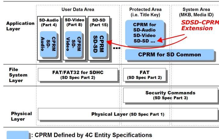
The *SDSD-CPRM* implementation uses one Media Key Block for all content types. Each content type has an associated profile. Currently, three profiles are approved or under consideration. Those include **SD-SD Audio**, **SD-SD Video**, and **SD-SD ePublish**. These profiles define the implementation of CPRM used to encrypt a specific type of content. Additionally, key management uses CPRM to generate and encrypt the keys. See [Figure 3 on page 6](#).
