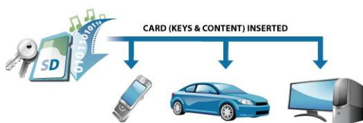
**Scenario 2:** Keys for the content, Key Library, reside on an SD Memory Card. The SD Memory Card is inserted into the *SDSD-CPRM* device. The receiving device has the encrypted content or has access to it from another source (HDD, PC, LAN, Mobile, etc.).
