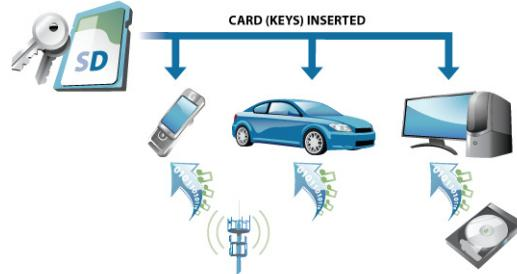
**Scenario 3:** Encrypted content and associated keys reside on an SD Memory Card. The SD card is inserted into the *SDSD-CPRM* device where it transfers the content and keys to the embedded SD memory. The SD Card is now removable.
