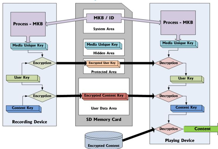
Toshiba Corporation's MQbic™ Digital Rights Management System is an example of a key management system for SDSD-CPRM.
