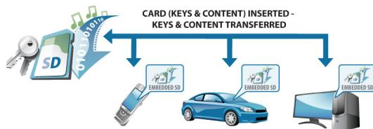
**Scenario 4:** Keys for the content, Key Library, reside on an SD Memory Card. The SD card is inserted then transfers the keys to the *SDSD-CPRM* device with embedded SD memory. The receiving device has the encrypted content or accesses it from another source (HDD, PC, LAN, Mobile, etc.). At this point, the SD Memory Card is removable.
